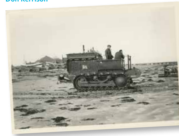
Above: The lifeboat launching tractor, with Boulmer village and pub in the background
