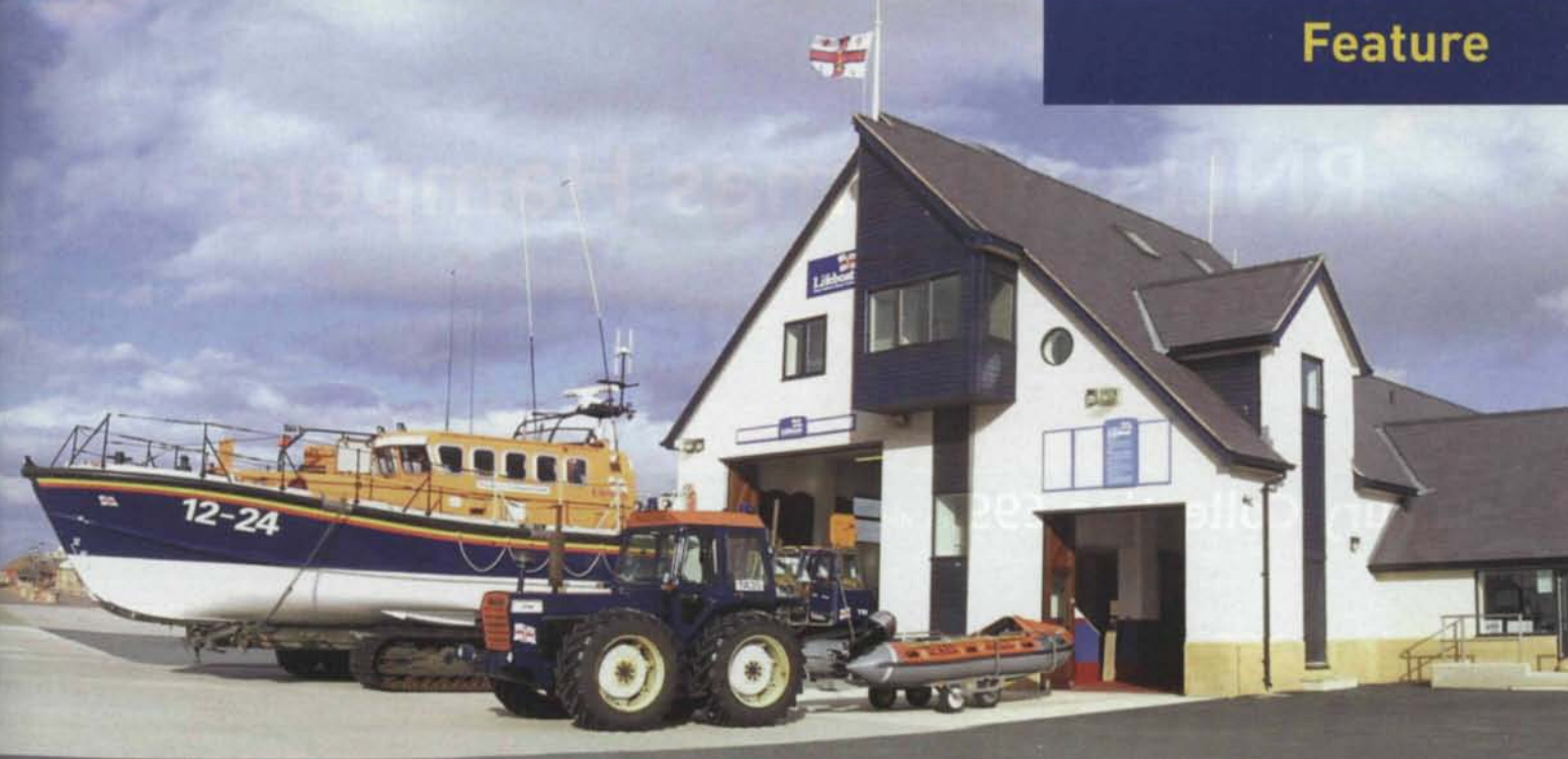
Rhyl lifeboat station houses a Mersey class all weather lifeboat, launched using a tracked carriage and tractor, and a D class inshore lifeboat, launched using a trolley and tractor. See page 17 for an example of an Atlantic 75 and carriage
