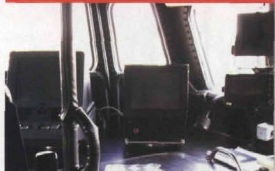
Above: The navigator's position on a Severn class lifeboat (screens left to right are: radar, chart plotter and depth log above the GPS)
