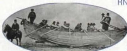
Zetland, the oldest surviving lifeboat, is of the Greathead type and was built in 1800
