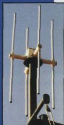
(Above) The masthead-mounted VHFDF aerial on a Trent
