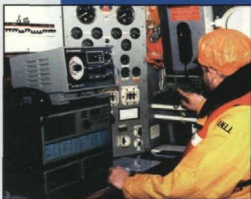
(Left) The MF receiver and transmitter are near the crew member's left hand with the MF DF set above. The much smaller VHF radio is by the crew's right hand
