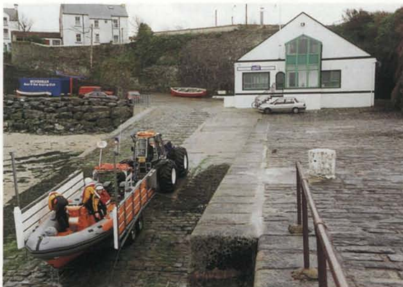
Above: Bundoran's Atlantic 75 lifeboat, Helene , is recovered by tractor and DoDo trolley after a launch.
