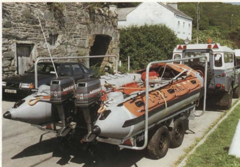
Above: Clifden's D class lifeboat can launch from several different sites using a Land Rover and trailer for launch and recovery.
