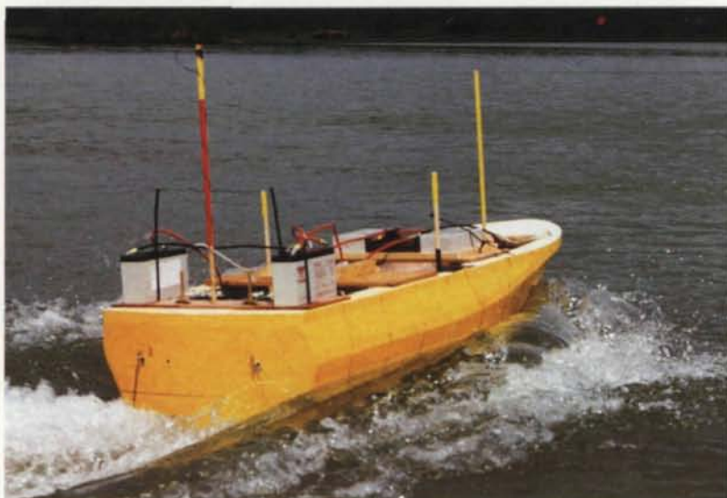
Some of the tank test models for the new Fast Slipway Boat were converted for free-running, radio controlled handling and manoeuvrability trials
