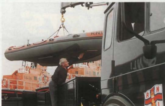
The truck's four-tonne crane makes the task of loading and unloading inshore lifeboats and other heavy equipment a one-man-job.
