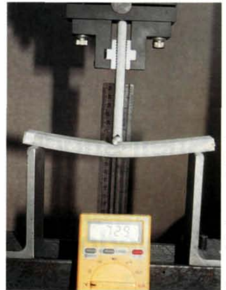
The test rig flexing a sample. This degree of flex was repeated up to one million times.
