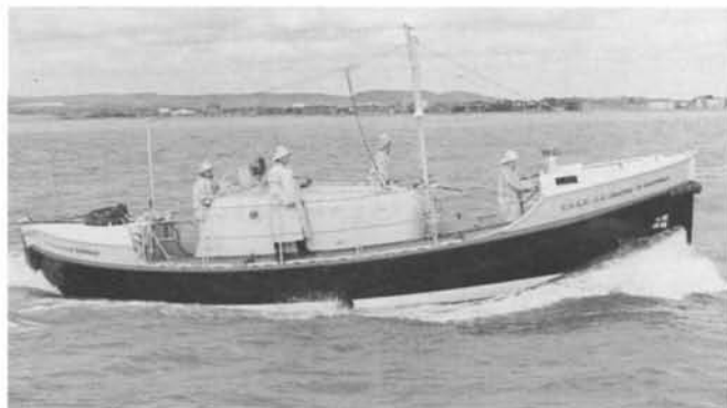
Initially the 37ft Oakley had a completely open cockpit (left, below) but the class was later equipped with a folding wheelshelter (below, right) to provide protection. Radar was also added, the scanner folding down into the forward cockpit. Both structures needed to fold to enable the boats to fit existing boathouses.
