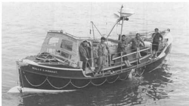
Initially the 37ft Oakley had a completely open cockpit (left, below) but the class was later equipped with a folding wheelshelter (below, right) to provide protection. Radar was also added, the scanner folding down into the forward cockpit. Both structures needed to fold to enable the boats to fit existing boathouses.
