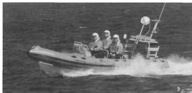
VHF transmitter/receivers are now very compact and can be fitted in boats as small as the RNLI's D class inflatables. This photograph of the first Atlantic 75 rigid inflatable clearly shows the aerial mounted on the mast aft – as high as practicable.
