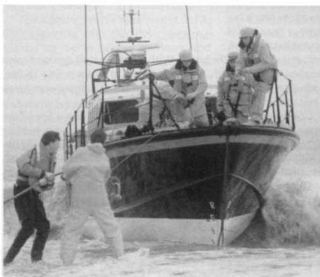
When a new carriage-launch lifeboat arrives at her station she is immediately re-launched and then recovered again as a final check on the carriage, tractor and lifeboat and to familiarise the shorehelpers with the new equipment. Recovery and launching
