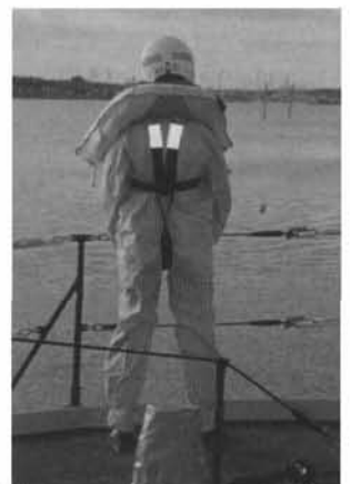
(Below) Rear view of the jacket, showing the retro reflective tape on its safety harness
