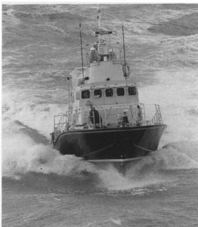
The high superstructure of an Arun class lifeboat may make her look 'top heavy' to some eyes, but is the key to her ultimate stability and safety.
