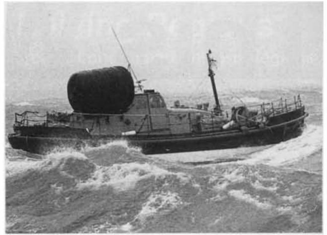
An effective but less elegant self-righting method. Inflating an air-bag, seen here on a 52ft Barnett, moves the centre of buoyancy to right the boat, but its bulk is less than convenient if left inflated.
