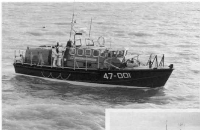
Two views illustrating the change in sheer between the two prototypes and the later production boats. 47-001 City of London (above) has the small 'kick' in the sheer to accommodate the steeper deck camber and false side deck - see text - while the production boats (right) have less camber and no raised section.
