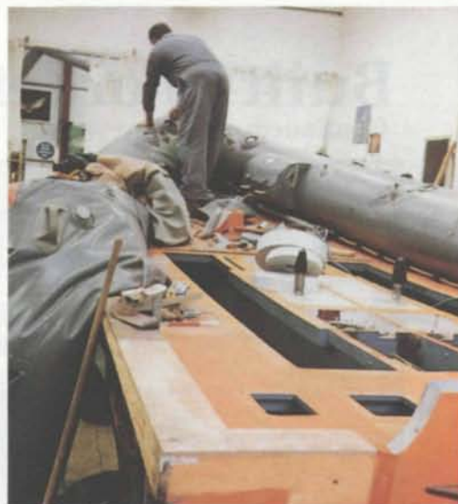
Above: Attaching the inflatable tubes to the Atlantic 21 hull. Surprisingly perhaps, the service life of tubes tends to be greater than that of the hull. Below: The Atlantic 21 in action - Southend-on-Sea's Percy Garon II . Photo A. McDougall, Evening Standard
