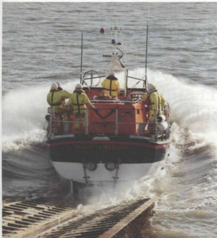
The need for fully protected propellers and rudders is obvious in this photograph of Selsey's Tyne class lifeboat leaving her slipway. Note the deep skeg just visible on the port side.
