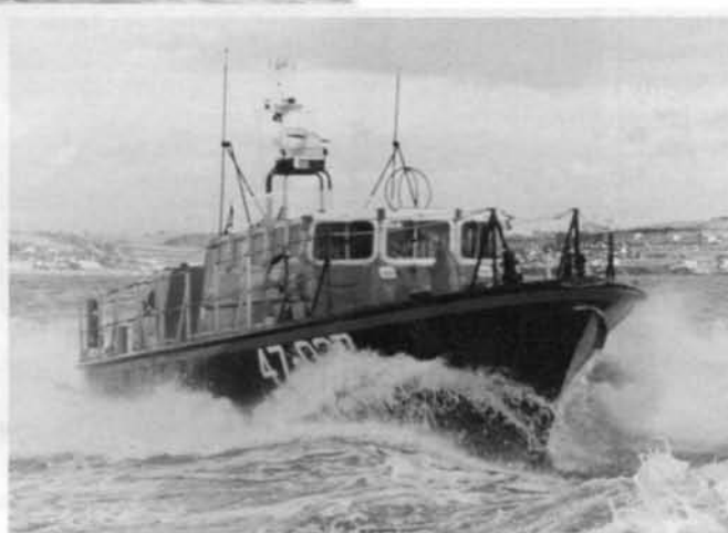
Two views illustrating the change in sheer between the two prototypes and the later production boats. 47-001 City of London (above) has the small 'kick' in the sheer to accommodate the steeper deck camber and false side deck - see text - while the production boats (right) have less camber and no raised section.
