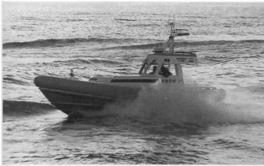
Left. The Dutch have developed a 10.6m rigid inflatable which has been in service since October 1990. The Valentijn class is jet powered and steered by 'buckets' over the outlets. She has been designed specifically for the shallow waters around the Dutch coast. A special hydraulic launching carriage has been developed which lifts the lifeboat into the correct position for launching.
