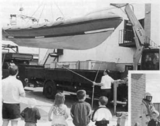
Above. Loading the RNLI's Mercedes 'road train'. Driver George Dadson demonstrates how an Atlantic 21 can be loaded single-handed with the hydraulic crane.
