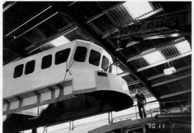
(Above). The unpainted wheelhouse module (also in FRC) is craned into position on the hull.
