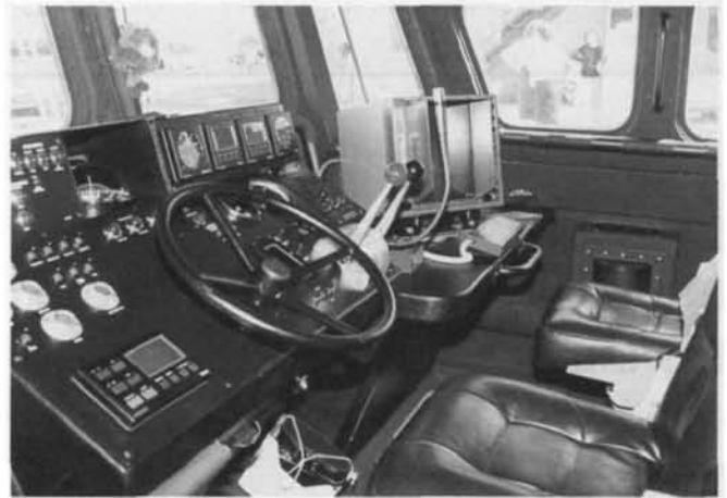
'Sprite', the lifeboat's mascot (provided by Osbornes for all lifeboats built by the yard) watches over the inside steering position with its engine controls and electronics.
