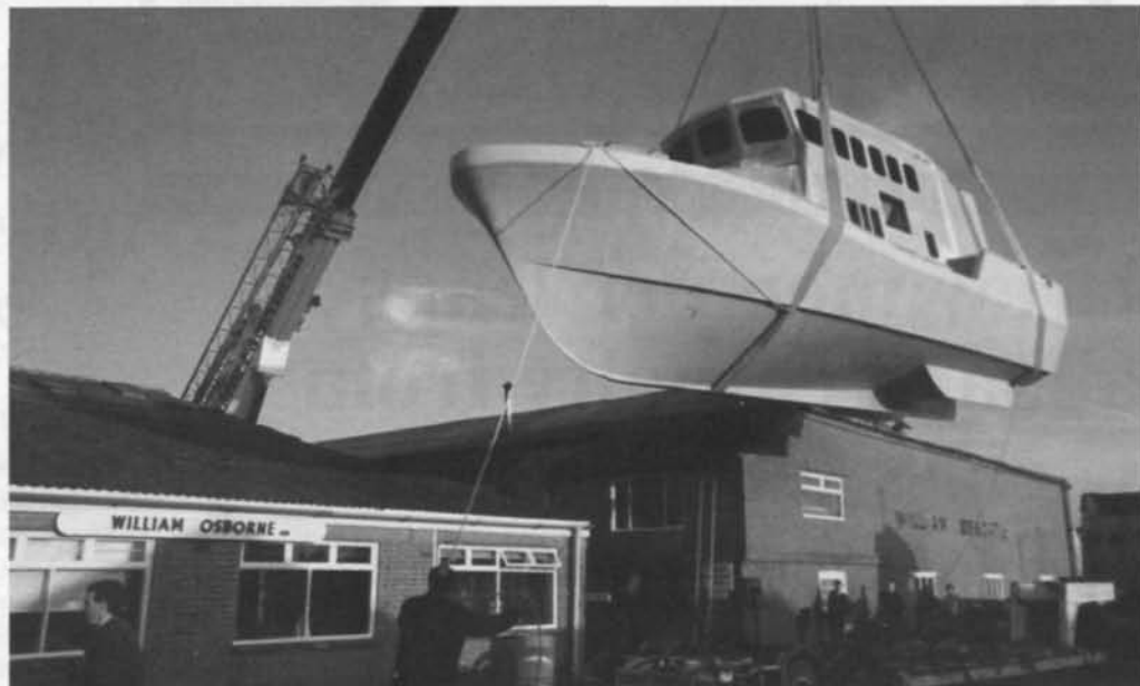
The hull and deck assembly of the prototype FAB 4 is hoisted into William Osborne's yard at Littlehampton for fitting out.
