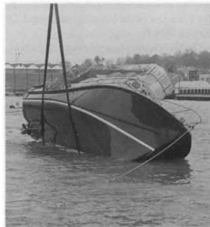
The hull form of the Arun class is shown clearly in this self-righting trial. Note the flat sections aft to promote planing and the small tunnels to allow larger propellers.
