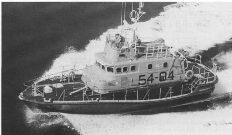
Tony Vandervell , the fourth Arun to be built (1976) was the first in GRP and the second to feature the extended stern which increased the length to 54ft overall. The wheelhouse is also GRP, although later boats reverted to aluminium.
