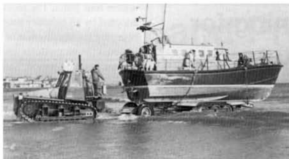
The hull shape must also provide full protection for the propellers, be suitable for launching and recovery from a carriage and light enough to be handled when ashore. (Photo Jeff Morris)
