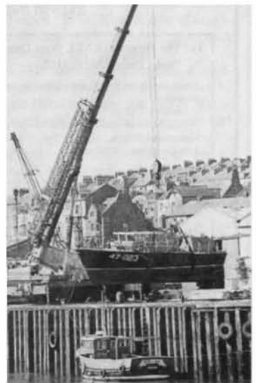
(Right) Whitby's Tyne class lifeboat City of Sheffield is pictured ready for her hull inspection and scrub down at the town's Endeavour Wharf. The operation took some three hours, but the lifeboat remained operational as she could have been re-launched at any time. (Photo courtesy Whitby Gazette,
