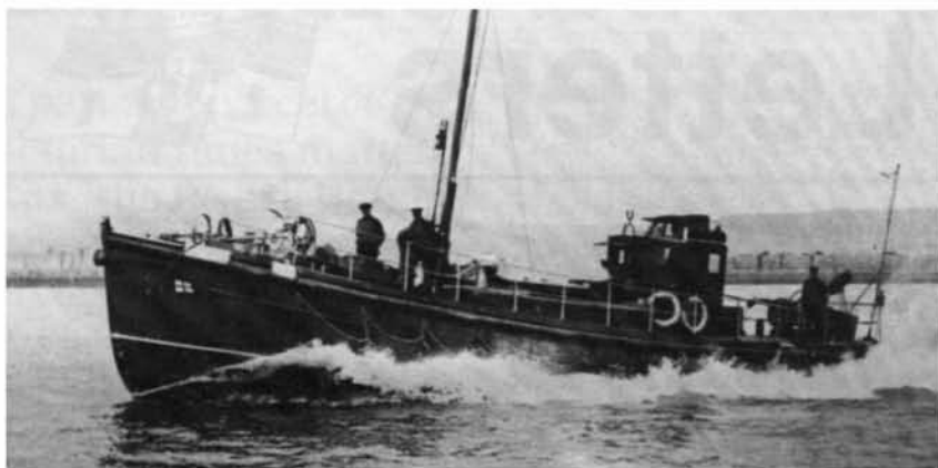
The Sir William Hillary to which Mr Hills refers below was the RNLI's first 'fast' lifeboat. Designed largely for rapid response in the event of an aircraft crash, she was 64ft long and powered by two 375hp petrol engines giving a speed of between 17 and 18 knots. She entered service shortly before the Second World War, and no other boat of her kind was built by the RNLI.
