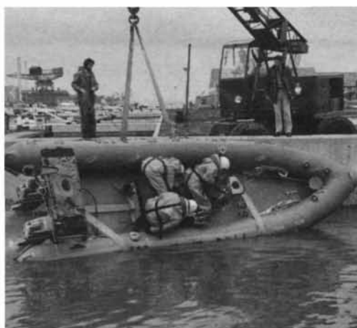
Above left. Crews are tipped into the River Medina twice during their courses to familiarise themselves with the righting procedures. A crane is used to capsize the boats.
