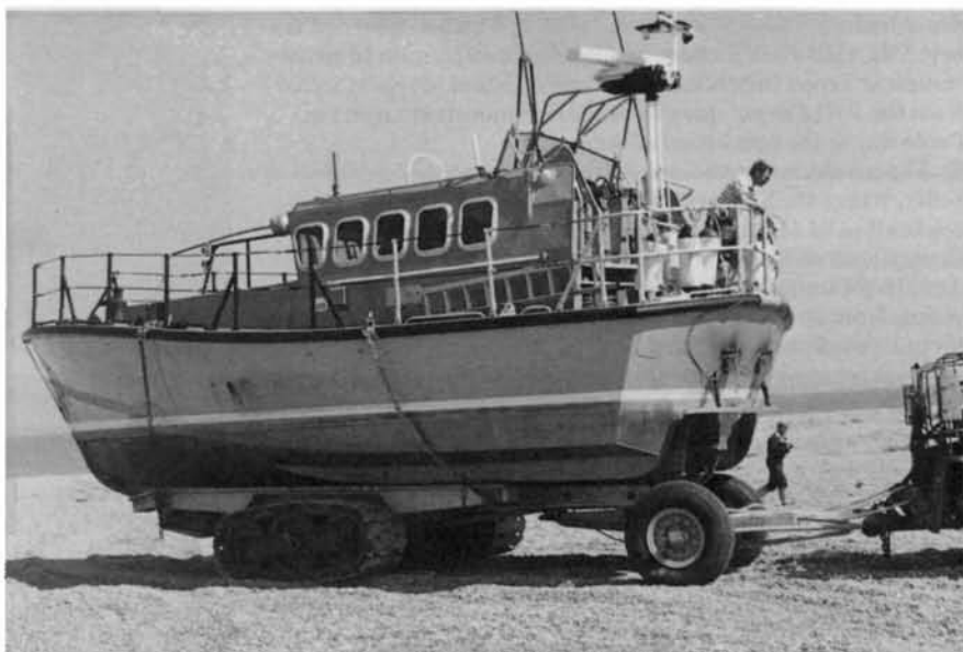
Pictured here, the production prototype of the RNLI's proposed fast carriage-launched lifeboat is currently undergoing extensive technical and operational trials, as part of its continuing evaluation. It is anticipated that the trials will be concluded during the early part of 1988.
