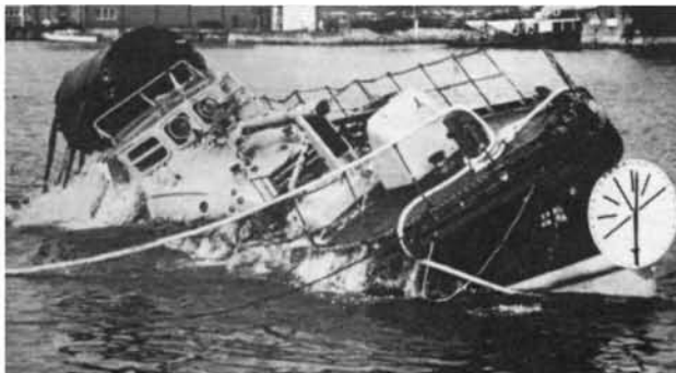
Sir Godfrey Baring, Workington's 46ft Watson lifeboat, recovering from capsize in trials after she had been fitted with an air bag to give her a self-righting capability.
