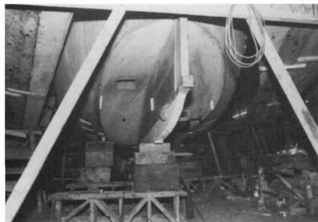
Fig. 2: After end jacked up so that holes can be drilled through deadwood for keel bolts, the longest bolt being 3ft 6in.
