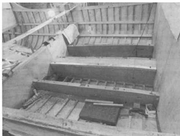
Fig. 2: Engine beds in place. Note bulkhead at forward end of engine room (right).
