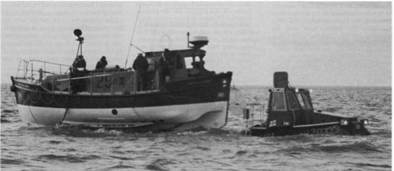
Hoyle lifeboat, Mary Gabriel, is pushed on her carriage before a launch.
