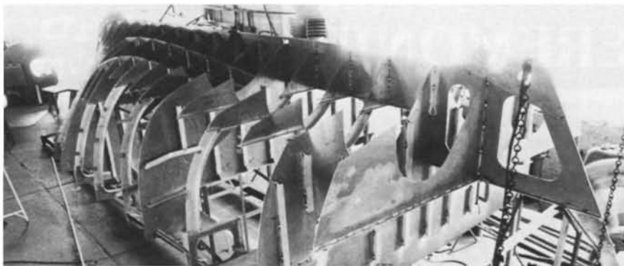
The hull's shape emerges. At this stage the boat is built upside down.
