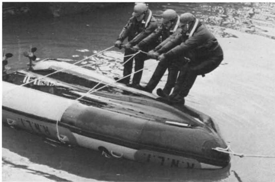
Three men not in a boat: should the twin-engined 17ft 6in C class inflatable lifeboat ever have the misfortune to capsize, this is the correct way to right her. The demonstration, given by RNLI staff at Cowes base, shows how the special righting gear, fitted to every C class inflatable, is put to use.
