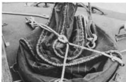
On deck and below, every piece of equipment is provided with its own place and with fastenings to keep it secure, even if the lifeboat is capsized. Fig. 2 (above): A drogue lashed down in its housing on the after deck of a Rother , and . . .
