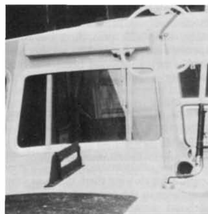
Fig. 7: Emergency low profile slot aerial, less vulnerable than the main aerial, mounted on the engine casing of a Rother class lifeboat.
