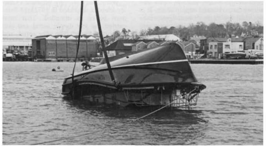
Fig 5: An Arun lifeboat inverted during her self-righting trials. Note how high she rides on her wheelhouse. A limited area in the centre of the boat, the 'envelope', will always be clear of the static water level.
