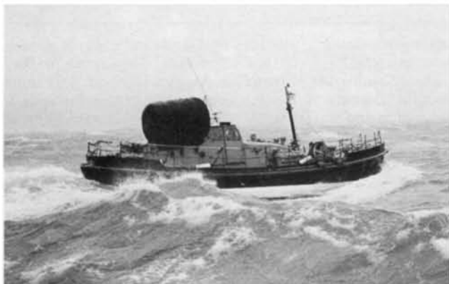
Salcombe's 47ft Watson lifeboat The Baltic Exchange (below, photograph by courtesy of Torbay lifeboat crew), and Barra Island's 52ft Barnett R. A. Colby Cubbin No 3 (below right, photograph by courtesy of HMS Gannett) are fitted with emergency air bags to give
