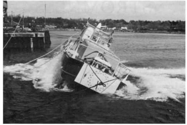
The 50ft Thames lifeboat, like Islay's Helmut Schroder of Dunlossit, is designed with a substantial watertight deckhouse to give her a righting capability. On her righting trials, once the strop is released she comes upright, shaking off the water.
