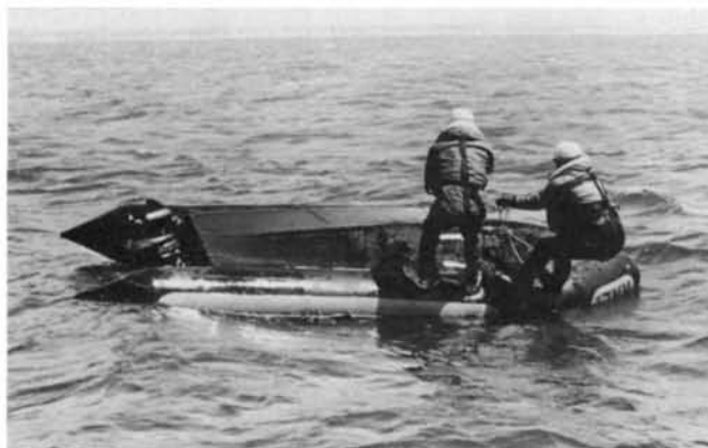
A righting drill, for use after capsize, has now been established for the D class inflatable lifeboat. Briefly, the crew climb on to the upturned boat, secure the painter to the lifting handles on the weather side, then stand on the lee side and, use their weight to parbuckle the boat over.
