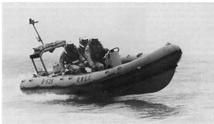
Atlantic 21 rigid inflatable lifeboat B539 is stationed at Brighton. Note that her helmsman is steering with his left hand, keeping his right on the throttles.
