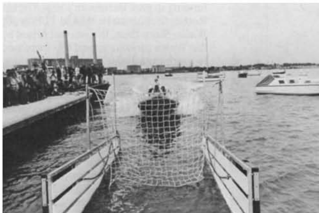
(Above, left and right) Demonstration recovery of the Atlantic 21 rigid inflatable lifeboat into her trolley mobile 'dock'.
