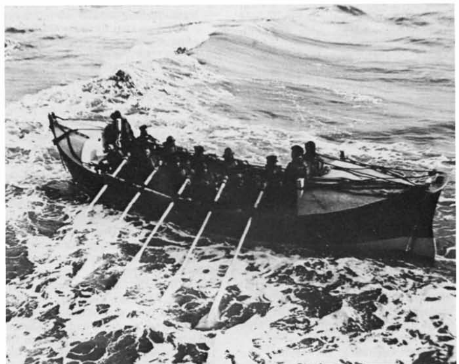
(Below) Selsey lifeboat John and Henry Skynner was built in 1885 and took part in the London Lord Mayor's Show of that year before going on station. She was 35ft long, 7ft 6in beam, pulled ten oars and was fitted with water ballast tanks.
