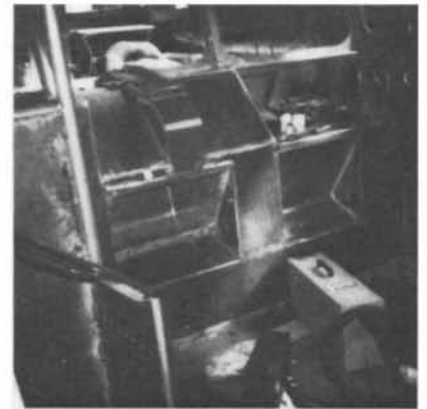
Fig 4: Coxswain's instrument console in place at forward end of wheelhouse ready to receive steering wheel and instruments (left) and radar display unit (right). Seats for coxswain and navigator will be fitted aft of the console in the lower part of which can be seen the foot rests.
