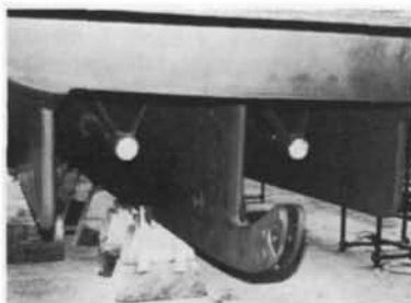
Fig 5 (below): The twin rudders are of fabricated mild steel, with steel stocks sprayed with stainless steel in way of the bearing surfaces.
