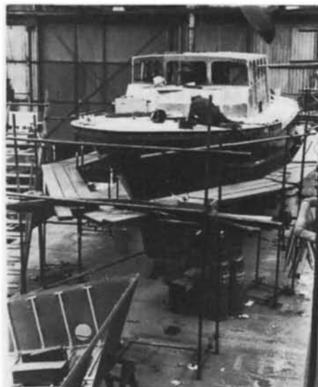
Fig 3 (left): The first FSB prototype fitted with aluminium alloy decks and wheelhouse. The after cabin superstructure, also aluminium, can be seen waiting in foreground.
