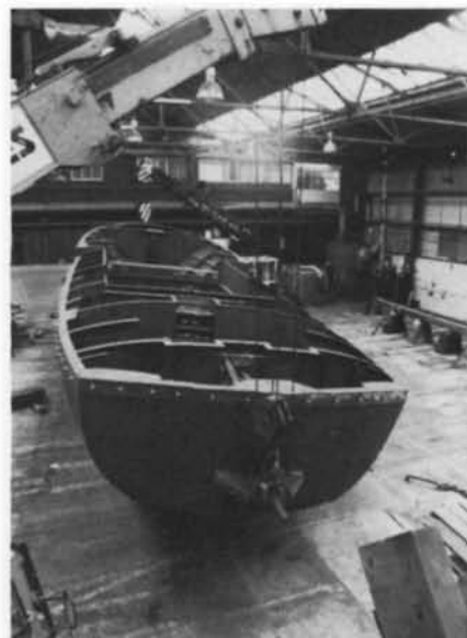
Fig 5 (below): The twin rudders are of fabricated mild steel, with steel stocks sprayed with stainless steel in way of the bearing surfaces.
