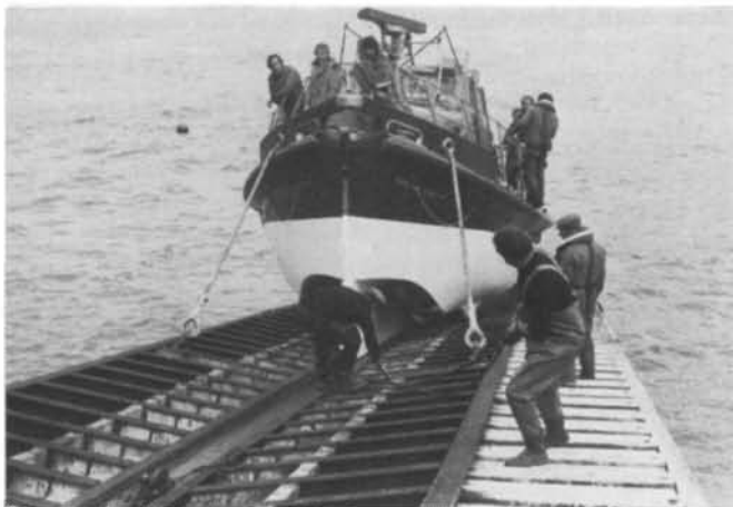
Once the lifeboat is high and dry, quarter stoppers support her entire 32 tons as the bridle is dismantled . . .
