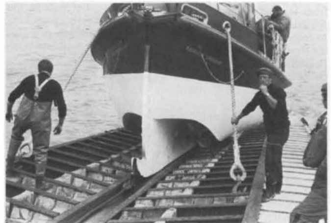
. . . the winch takes the weight, the quarter stoppers are removed and steadily the lifeboat is hauled up the slipway.
