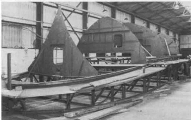
Fig 3: (right) Building starts of the first 47ft steel fast slipway lifeboat prototype. The gunwale is laid down on a deck jig and the five watertight bulkheads and transom erected.
