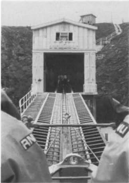
Winchman Ernie Bennett activates the winch which, with a V-shaped bridle of special flexible wire, hauls the lifeboat clear of the water.
