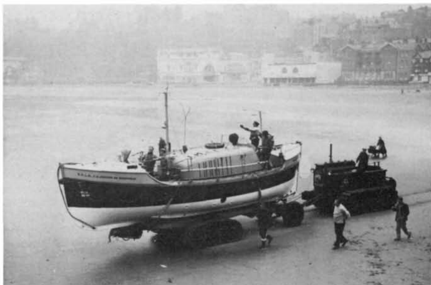
The 37ft Oakley, designed by R. A. Oakley, the Institution's surveyor of lifeboats, was the first modern lifeboat with a self-righting capability, and the first boat of the class to be built. J. G. Graves of Sheffield, went on station at Scarborough in 1958. Her self-righting ability is provided by water ballast transferring, should the boat be knocked down, from a bilge tank into a righting tank on her port side. All modern lifeboats undergo righting trials in controlled conditions, being hauled over by crane, before being sent to station.
