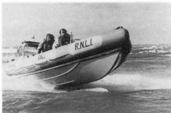
The Atlantic 21 rigid inflatable, powered with twin outboard engines and attaining a speed of 30 knots, first went on station at Hartlepool in 1972. Smaller, inflatable lifeboats were introduced into the RNLI fleet in the 1960s.
