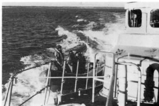
Easing in between the bow and stern waves of Yarmouth's 52ft Arun to run alongside at about 14 knots: a demanding exercise which is invaluable in training the helmsman to steer with one hand only, leaving the other for the throttles.
