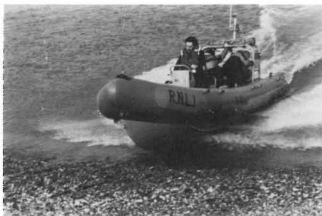
Practising beaching, to land well clear of possible breaking waves or heavy surf: as the helmsman brings the Atlantic 21 lifeboat in at speed the two crew members prepare to tilt up the outboard engines clear of the ground.
