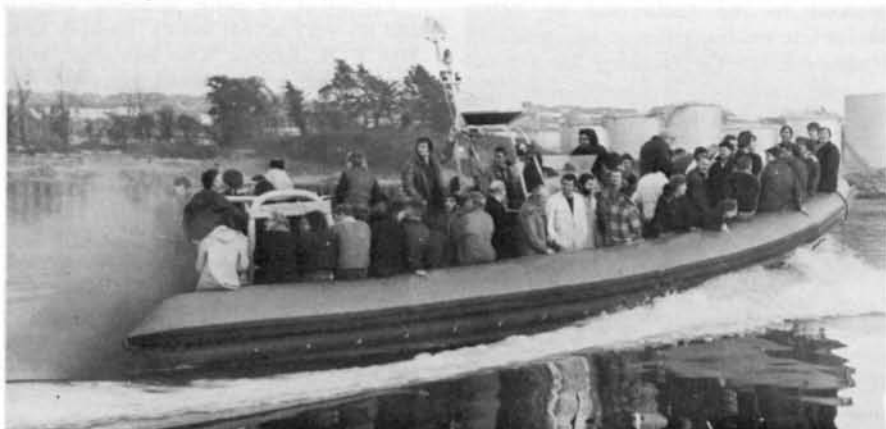
The prototype RNLI Medina 35, Mountbatten of Burma, on trials at Cowes. The more people on board, the greater her stability.
