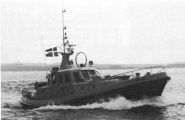
Denmark: (below, left) A 15.2m self-righting lifeboat stationed on the west coast of Jutland. Finland: (below, right) The 20.5m steel Harmaja built to work in ice is one of the Finnish Lifeboat Society's largest rescue cruisers.
