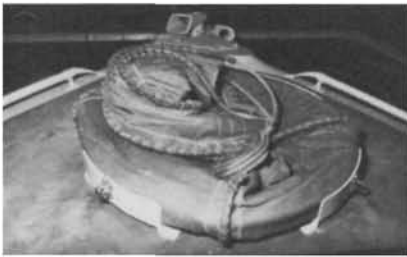
After deck stowage for drogue and, at stern (port), drogue fairlead. Rectangular bronze emergency tiller housing is mounted on steering gear box.
