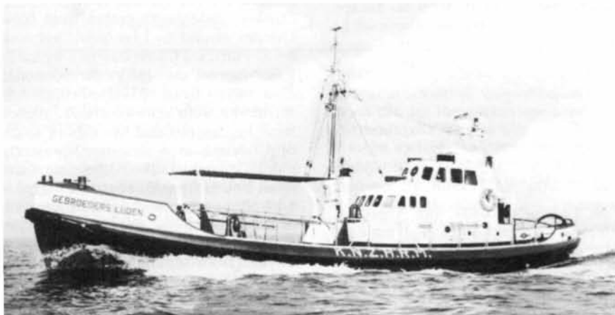
The Netherlands: (above) Gebroeders Luden, one of six 20.37m self-righting lifeboats in the KNZHRM fleet. (below) President Jan Lels, the oldest twin screw 'all weather' lifeboat in the KZHRM fleet.
