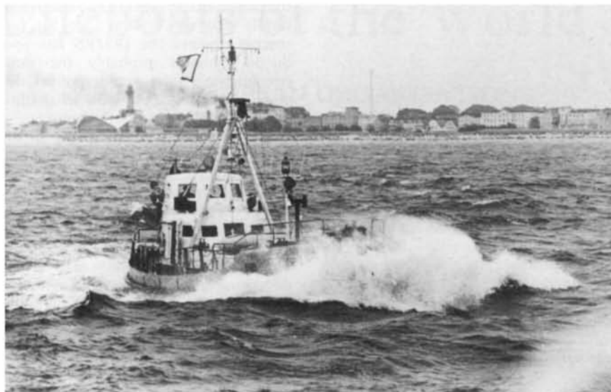
Democratic Republic of Germany: Poel is one of East Germany's 17.9m lifeboats; speed 10 knots. The service also has two rescue cruisers and inflatable inshore lifeboats.
