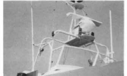
Fl Lt J. A. Cowan and Sergeant Dick Guy of RAF Brawdy were awarded the 1978 L. G. Groves Memorial Aircraft Safety Prize for their invention of the 'Brawdy Homer'. This instrument will enable ships to home on to any emergency locator transmitter used by people adrift in liferafts in the sea. Barry Dock's 52ft Arun helped with trials of the prototype and in this picture can be seen the twin aerials mounted one on each side of the radar platform.
