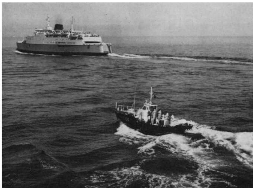
A 44-foot steel life-boat. A development of this U.S. Coast Guard life-boat, with a speed of 17 knots is destined for Falmouth. The R.N.L.I. has already six of the 44-foot version in service.
