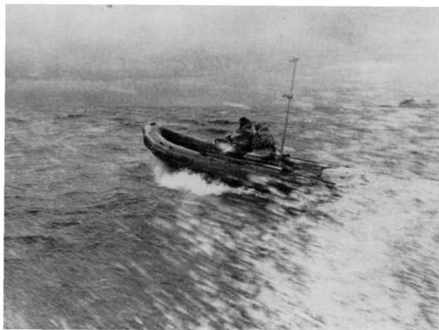
Inflatables were first introduced into service in 1962, and the current development is the Atlantic 21 rigid bottomed inshore rescue boat, here shown at speed.
