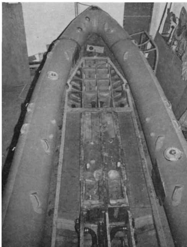
baffles of integral water ballast tanks. Hole of transom scoop can be seen on port side. (Right) Flexible neoprene pipes from manifold (inboard of transom) lead port and starboard to water ballast tanks and forward, on port side of centreline, to trim tanks via a Y piece.
