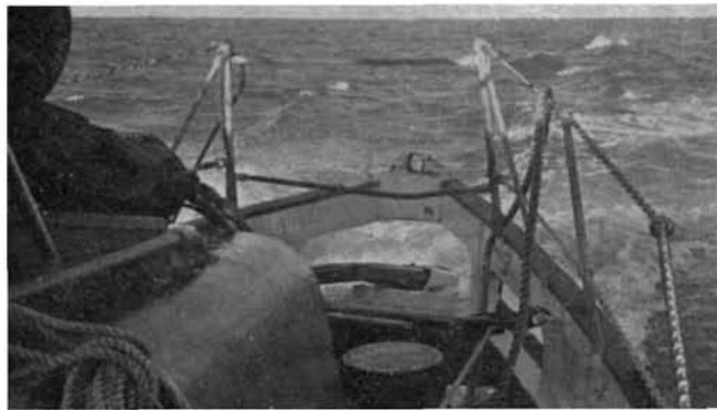
Emergency steering: the tiller can be seen on the rudder post.
