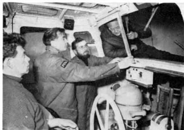
37' Oakley lifeboat James and Catherine Macfarlane, back in Padstow after her service of December 7. (l. to r.) Second Coxswain Trevor England, DI (SW) Lt.-Cdr. R. S. Portchmouth, Coxswain Anthony Warnock and Honorary Secretary Harry Lobb inspect damaged windscreen central stiffener; it was replaced by two upright strengthening bars spaced either side of the centreline.
