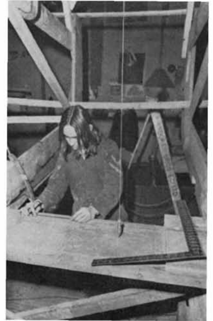
Measurements giving the fore and aft positions of all transverse members—moulds, bulkheads and timbers—are brought down from building batten to hog by plumb line.
