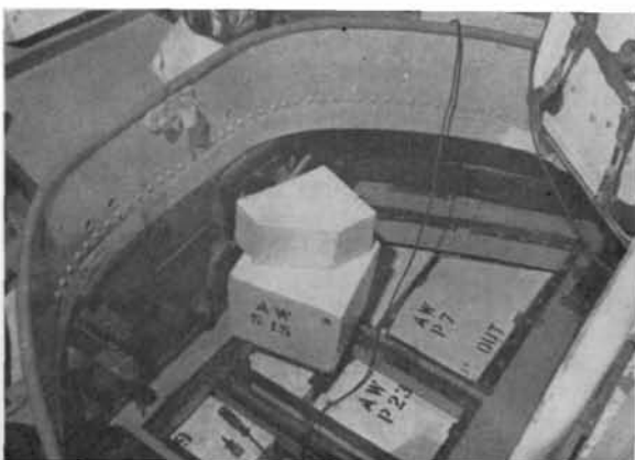
Fig. 3: Buoyancy air cases, each shaped to fit and marked with its position, are taken out when opening up the hull for examination at partial and complete survey...
