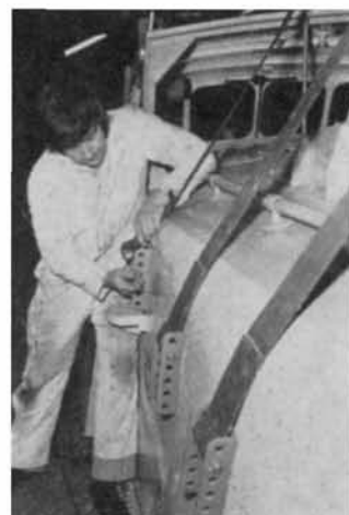
Fig. 5: (Right) Each end of the three securing straps are attached to brackets, bolted to cabin sides, with stainless steel retaining pins. Although brackets make allowance for six possible positions, it is normal to use the second from top holes.
