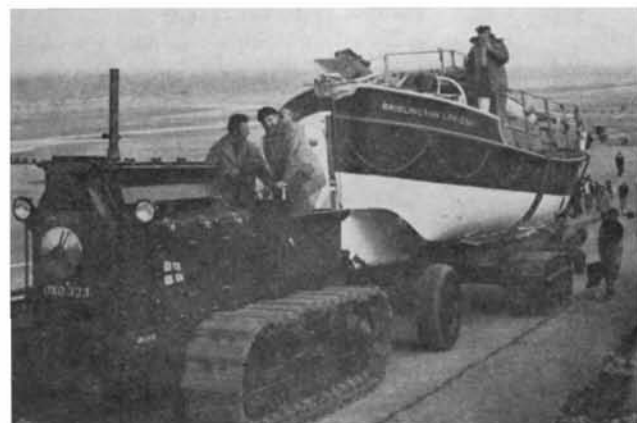
5: . . . channel track of little turntable (left) on which she can be swung round to convenient position for mounting on carriage. Tractor moves round carriage . . .
