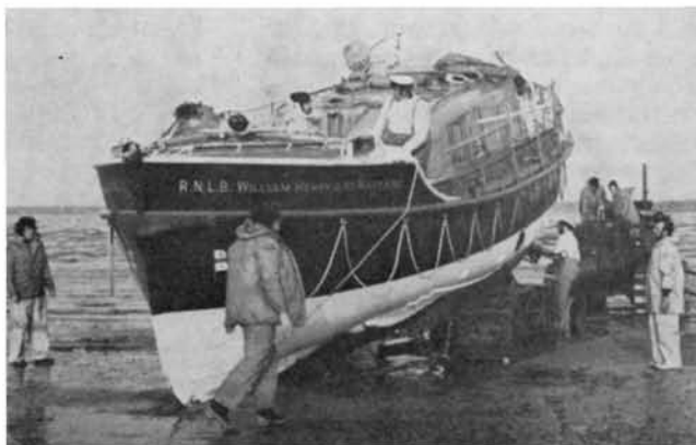
6: . . . and hauls boat on. Aligning of turntable with carriage is critical. Securing chain is rove through an after ruffle hole to prevent boat overriding carriage.
