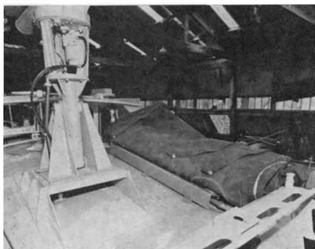
Fig. 3: (Left) Radar scanner has been moved to port of after cabin top, and air bag roof channel bolted in position to starboard. Note manifold leading under channel and, at its fore and aft ends, air inlets into bag.
