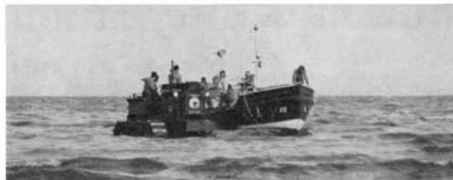
2: . . . receive from her crew a heaving line to bring wire through ruffle hole in boat's forefoot.
