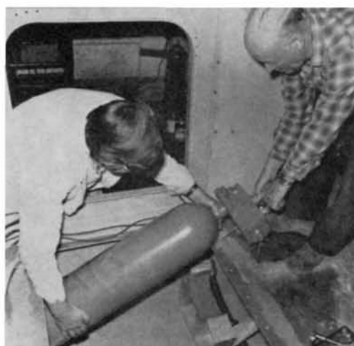
Fig. 1: Compressed air bottle, with pneumatic valve box at end, is lowered on to its mounting cradles by British Hovercraft conversion crew, Brian Augustus (left) and Leslie Harris. Note new square stretcher hatch into deck cabin, and stainless steel plate decking in old after-well.
