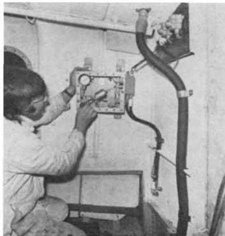
Fig. 6: Brian Augustus inspects anti-bounce device in control box. Weighted gravity sensitive lever can be seen in centre, pressure gauge on top left and a tube of silica gel crystals (to ensure there is no moisture in this watertight box) top right. Note high pressure hoses connected to control box (they will be connected through bulkhead to compressed air bottle valve), and larger diameter hose which connects air bottle to manifold in roof channel.
