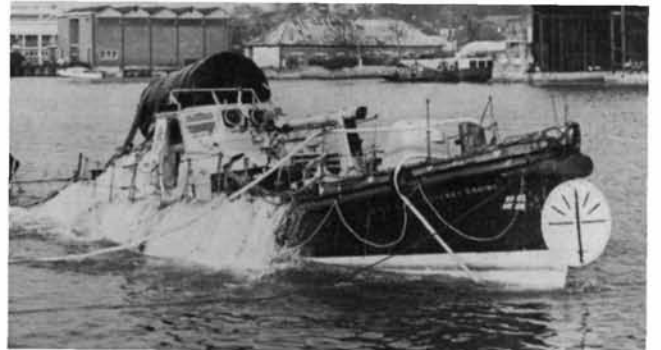
Air bags which, when inflated, will initiate righting are fitted to Atlantic 21 ILBs (right above), and to Watson and Barnett lifeboats (right)
