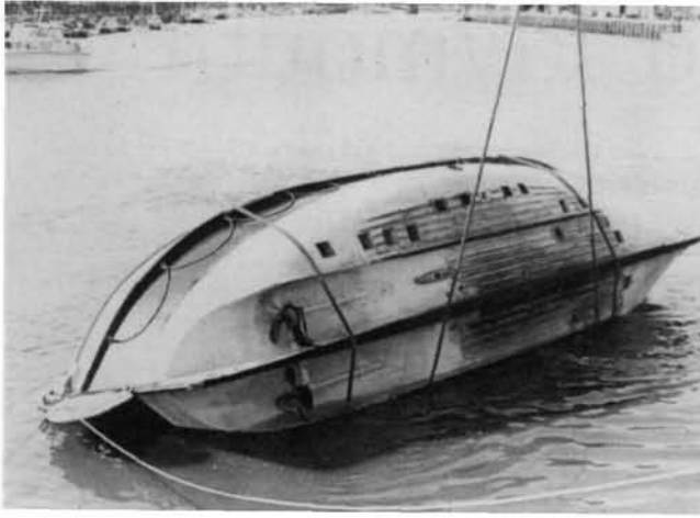
From 1851 the test of self-righting ability has been simple and thorough: 'Capsize the boat...
