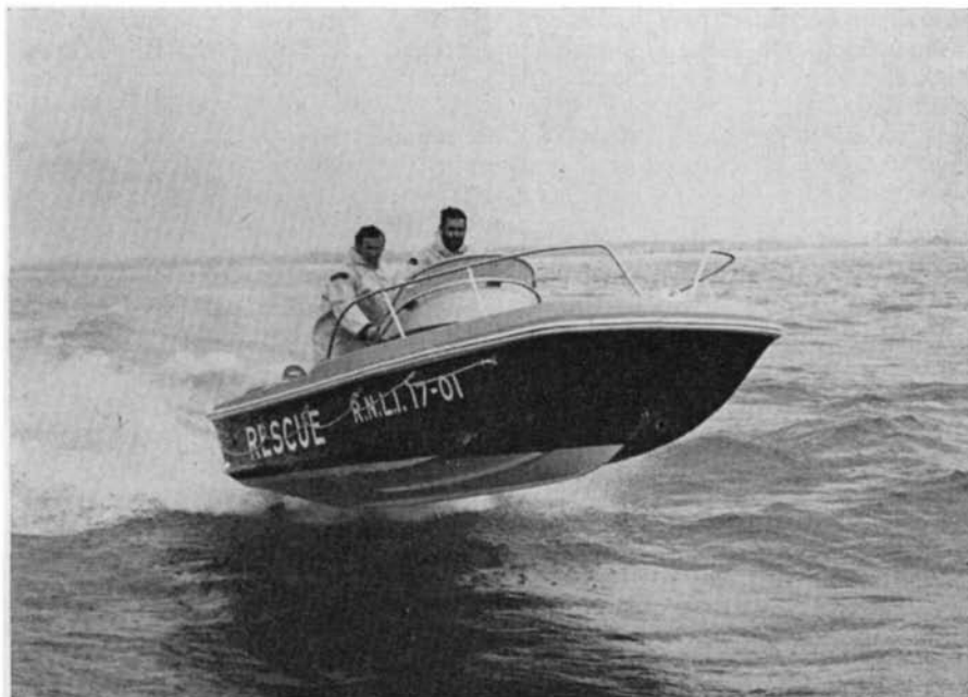
Pictured here is the first rescue boat with a fibre-glass hull to be tested under operational conditions by the R.N.L.I. It is a 17-foot dory built by Dell Quay Productions Ltd., at Itchenor, Sussex. (See pages 464 and 482.)
