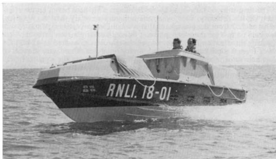
The Hatch boat (18-01), which was illustrated in The Life-boat for March, 1967, has been modified and is now self-righting. She can be used as a boarding boat to take life-boat crews from the shore to life-boats which remain afloat, and she can also be used for rescue purposes. Her self-righting capability was tested in May, 1968. In calm water she can reach a speed of up to 26 knots.
