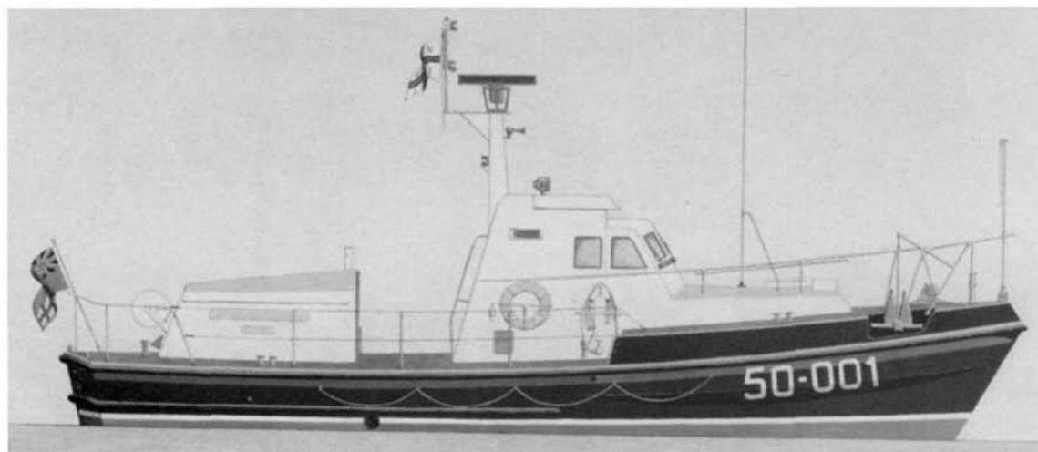
Of the 11 new life-boats ordered in 1971 four were of the 44-foot steel Waveney class, three of the 37-foot Mark II Rother (above), two of the 50-foot steel Thames (below), one of the 52-foot Mark II Arun and one of the 71-foot steel Clyde classes. The artist's impression of the 37-foot Mark II is provisional and the type will not carry all the antennae shown.
