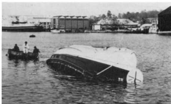
As reported on page 108, 46-foot 9-inch and 47-foot Watson class life-boats are being fitted with two self-inflatable bags which will bring them back to the upright position if they should capsize once. The pictures, beginning left with a tank test model being righted in this way, show the former Wick life-boat Sir Godfrey Baring under test. The pictures are reproduced by courtesy of British Hovercraft Corporation Ltd., East Cowes, Isle of Wight.
