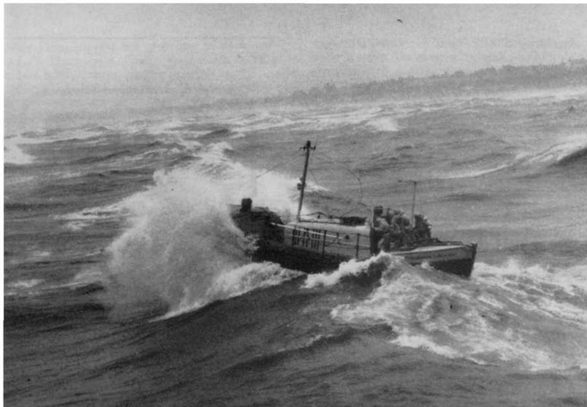
The Bridlington life-boat—a 37-ft Oakley self-righting type—heading into stormy weather. by courtesy of T. M. Carter
